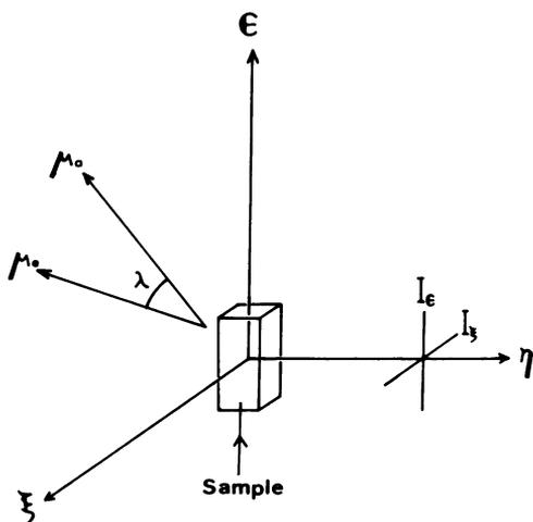
FIGURE 1 Geometry of the system. Excitation light is polarized in the direction of  $\epsilon$ . Fluorescence is observed along  $\eta$ . The two vectors  $\mu_a$  and  $\mu_e$  represent the directions of absorption and emission transition moments of a fluorophore in the sample.
