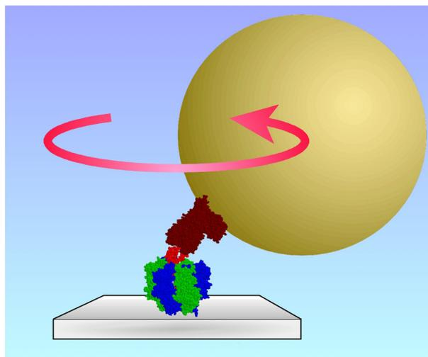
**Fig. 5.** *Imaging  $F_1$  rotation through a gold bead [2]. The  $\beta$  (green) subunits were fixed on a glass surface, and a 40-nm gold bead was attached to the central  $\gamma$  subunit (red) through streptavidin and BSA (brown) that served as glue. When the bead was attached obliquely as shown in the figure, rotation of the  $\gamma$  subunit resulted in a circular movement of the bead image. The rotation angle was estimated from the circular trajectory of the bead movement.*
